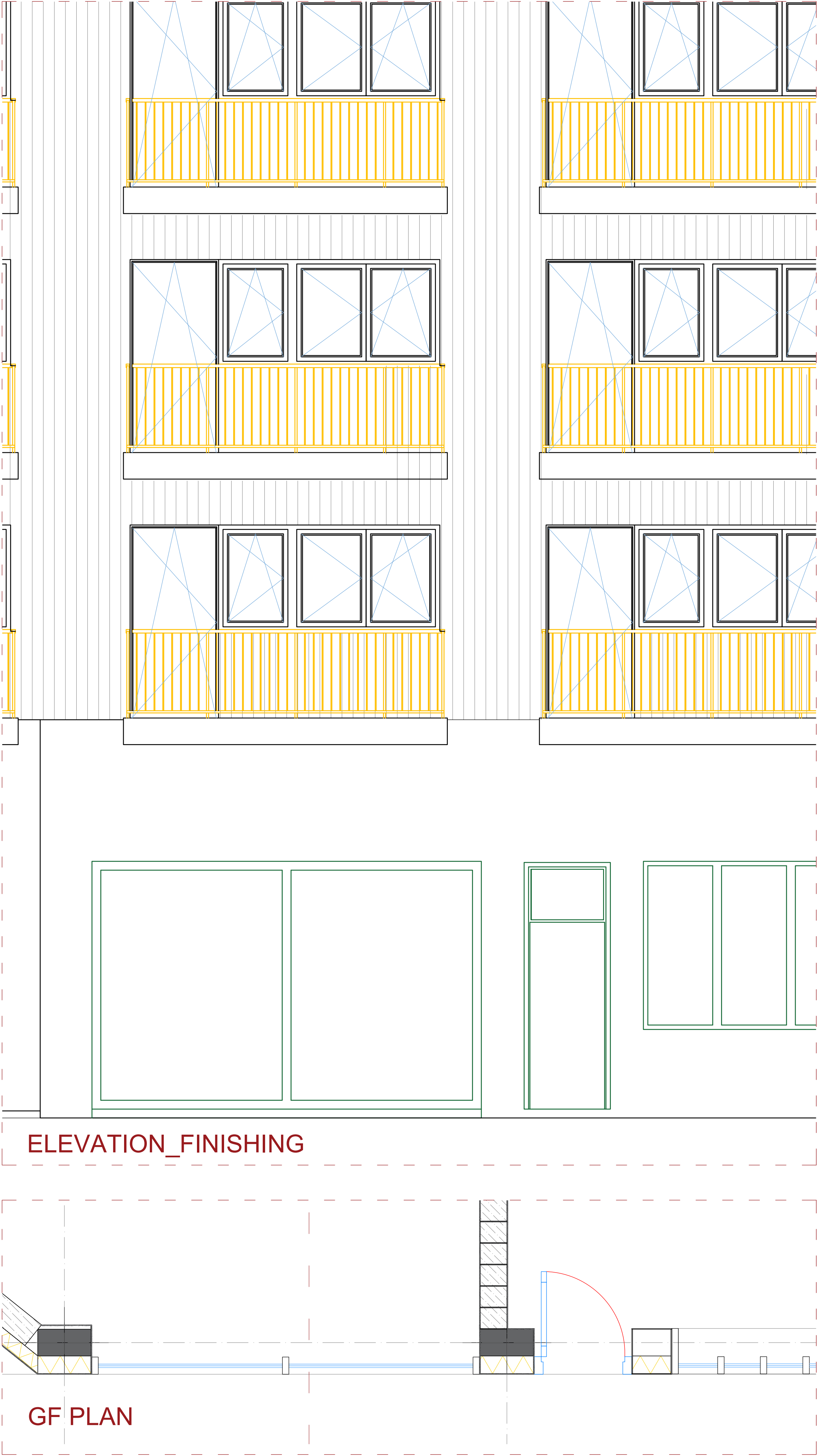
LUJZA UTCA ELEVATION — FACADE DETAIL — CORRUGATED METAL SHEET CLADDING
