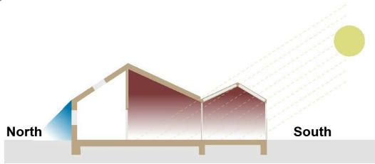
The glasshouse reduces heat loss from the main house as windows are protected from cooling wind and rain. This increases the insulation value of the southern facade by an additional ratio of 0.2. Combined with individually managed internal thermal curtains, the two layers add an additional ratio of 2, giving a total ratio of 4.2 for the southern facade at night.
